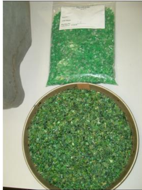
Photo 2: Flakes before and after oventest
