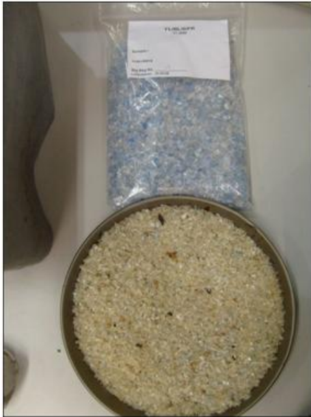
Photo 1: Flakes before and after oventest
