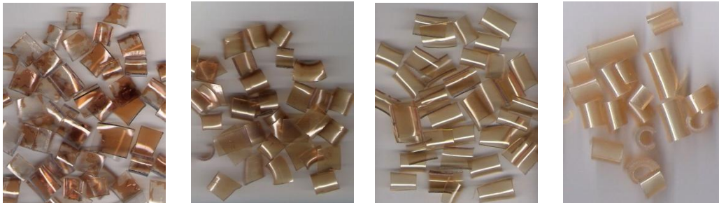
Photo 3-6: Discolouration in flakes after oventest
